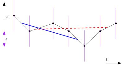
Figure 4. A 1-D trajectory with augmented vertices. The dashed shortcut is invalid because it does not intersect all augments between its start and end points. The other shortcut intersects the augments and is valid.
