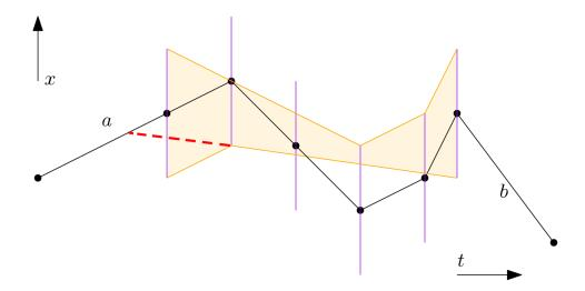
Figure 5. The hourglass consisting of two convex demi-hulls on the two sets of endpoints of the augments. Each demi-hull defines either the min or max function. If extending a segment of the demi-hull creates an intersection point with a (as can be seen with the dashed line), the value of  $\lambda$  at that point is a breaking value for that extreme function.
